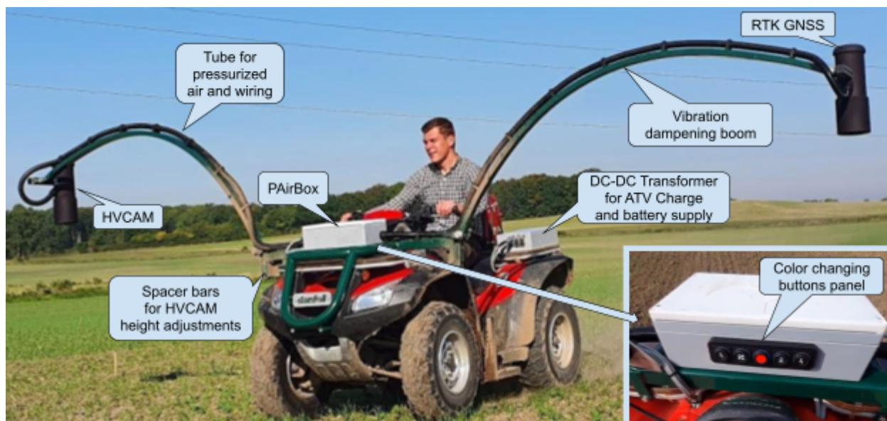
Figure 1: Overview of components in the Dual-HVCAM-system. Honda ATV including explanatory labels.
